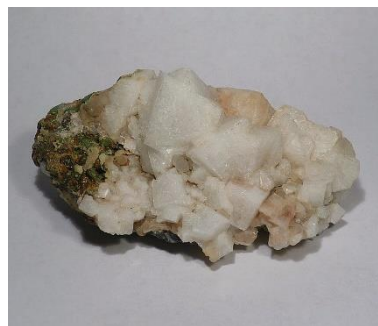
Abb. 6: Chabasit [3] \text{Ca}[\text{Al}_2\text{Si}_4\text{O}_{12}] \cdot 6\text{H}_2\text{O}
