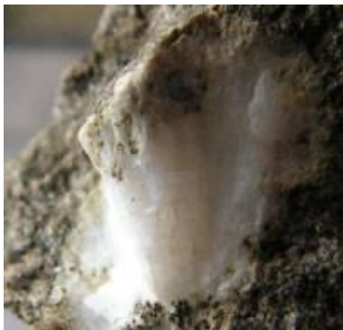
Abb. 5: Faujasit [2] \text{Na}_2\text{Ca}[\text{Al}_2\text{Si}_4\text{O}_{12}] \cdot \text{H}_2\text{O}
