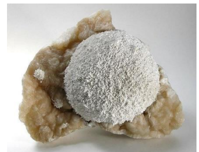
Abb. 7: Mordenit [4] \text{Na}_2[\text{Al}_2\text{Si}_{10}\text{O}_{24}] \cdot 7\text{H}_2\text{O}
